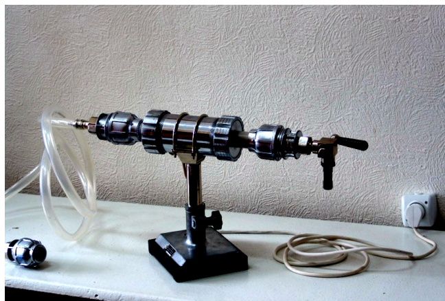
Fig. 3. Device of magnetic processing of food solutions (UMOPR)
